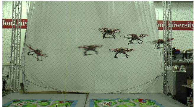
**Figure 27.** Overlay of snapshots showing the hexarotor executing a short segment of the random set of trajectories.
