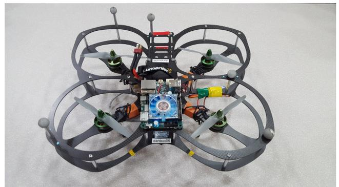
**Figure 6.** The quadrotor and ODROID-XU4 used for experimental validation of the Robust EPC algorithm.
