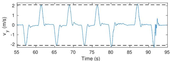
**Figure 29.** Velocity profile for the hexarotor applying (non-robust) EPC. The dashed lines indicate the constraint bounds.
