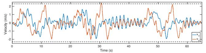
**Figure 19.** Velocity profile for the quadrotor applying Robust EPC along the circle trajectory in the high-wind scenario. The velocity obeys the constraint bound aside from one minor constraint violation of 0.09 m/s.
