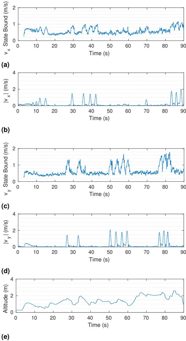
**Figure 28.** Constraint bounds on hexarotor  $x$ -velocity (a) and  $y$ -velocity (c) vary with the vehicle's current speed in each direction (b,d) and altitude (e), reflecting the changing uncertainty reported by visual odometry.
