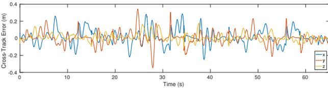
**Figure 20.** Cross-track error while the quadrotor executes the circle trajectory in the high-wind scenario is nearly zero-mean and shows some improvement over time.
