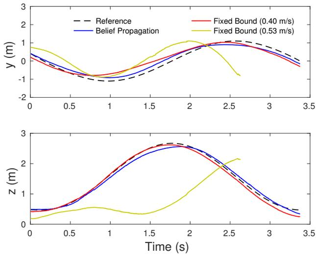
**Figure 14.** Quadrotor position along the  $y$ - and  $z$ -axes for Robust EPC and the fixed bound approach as compared to the reference trajectory. The fixed bound approach that uses the true upper bound (0.53 m/s) fails to track the trajectory. The mean and max error for Robust EPC along the  $y$ -axis are 0.22 and 0.41, respectively, while for the successful fixed bound approach (0.40 m/s), the mean and max error are 0.24 and 0.51.
