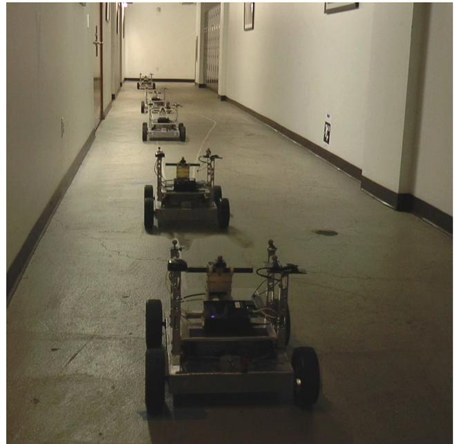
**Figure 23.** Overlaid video frames showing the ground robot tracking the trajectory through the long hallway via SLAM-based localization.
