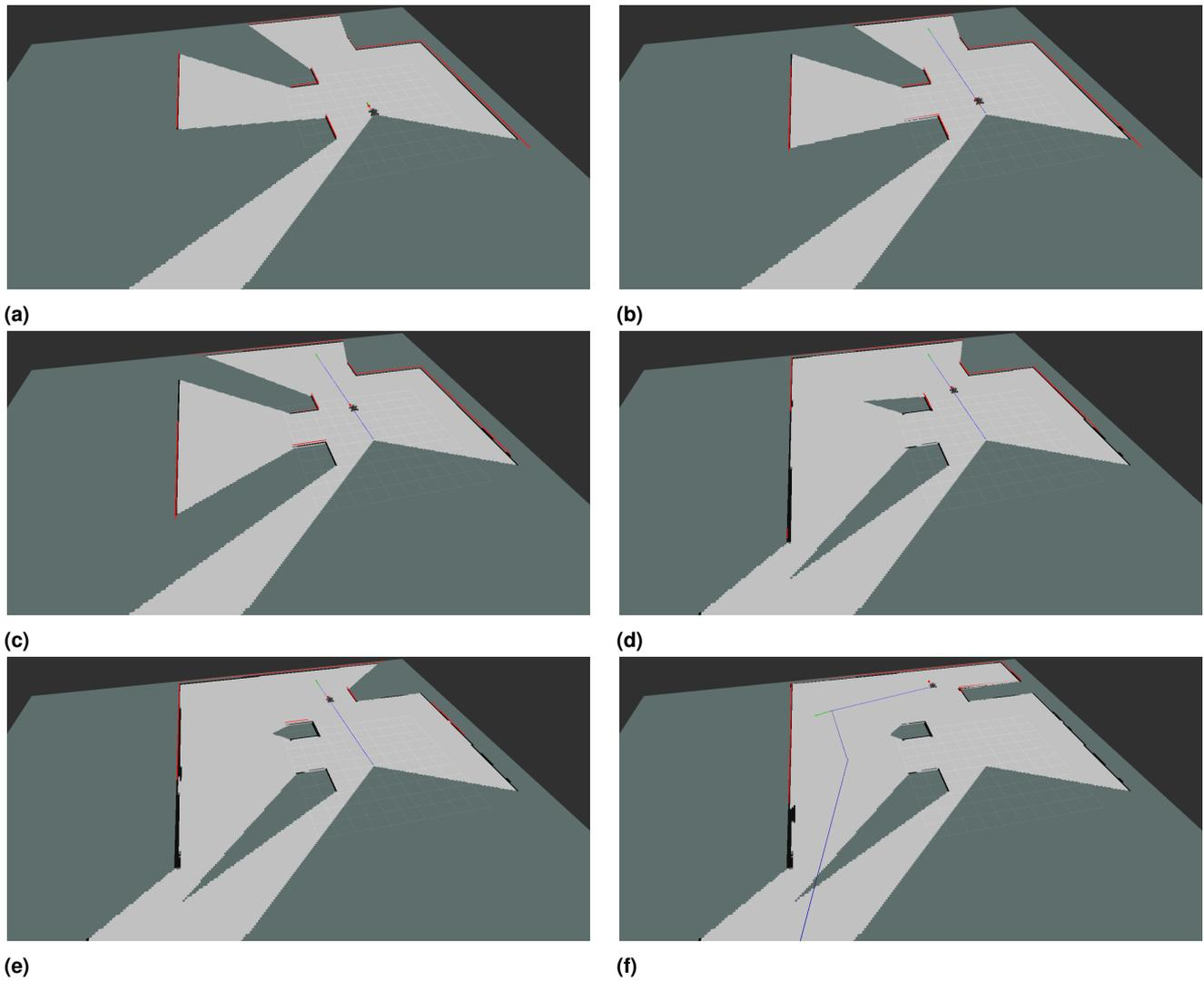
**Figure 3.** A series of snapshots showing a segment of the ground robot simulation trial. The blue lines denote the trajectory being tracked by the ground robot as it traverses the unknown environment. The successive frames illustrate the simulated laser scanner (red dots denote simulated laser returns) building a map of the environment that drives the localization subsystem.
