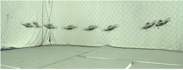
**Figure 7.** Snapshots of the quadrotor executing the linear trajectory.
