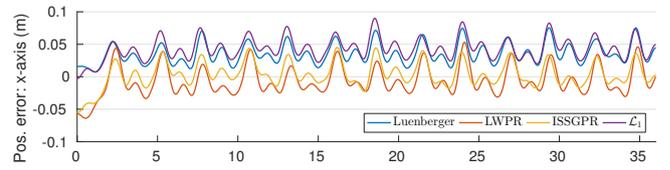
**Figure 8.** Cross-track error for quadrotor applying EPC with the three model adaptation strategies discussed and  $\mathcal{L}_1$  adaptive control. LWPR and ISSGPR yield superior tracking after gaining experience. To better visualize the low-frequency components, we apply exponential smoothing with a two-second window.
