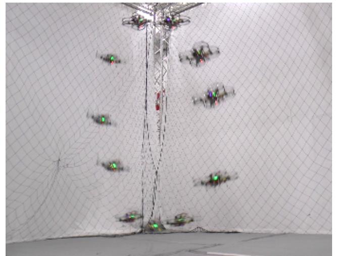
**Figure 13.** Quadrotor executing the vertical circle trajectory used to evaluate belief propagation.
