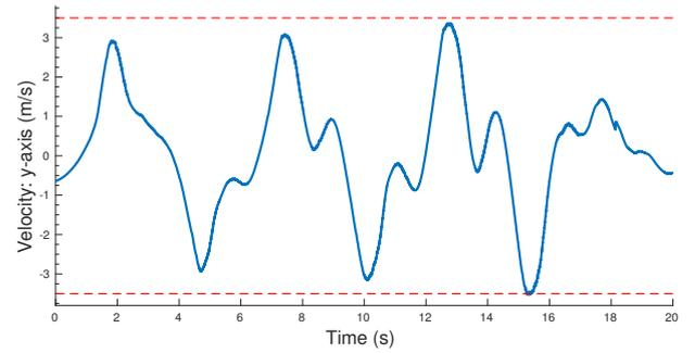
**Figure 16.** The quadrotor's velocity profile applying Robust EPC along a high-speed linear trajectory. There is a small constraint violation of 0.03 m/s during the last lap.
