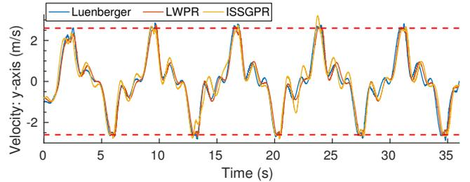
**Figure 9.** With injected noise, (non-robust) EPC yields velocity constraint violations for all three model adaptation strategies.
