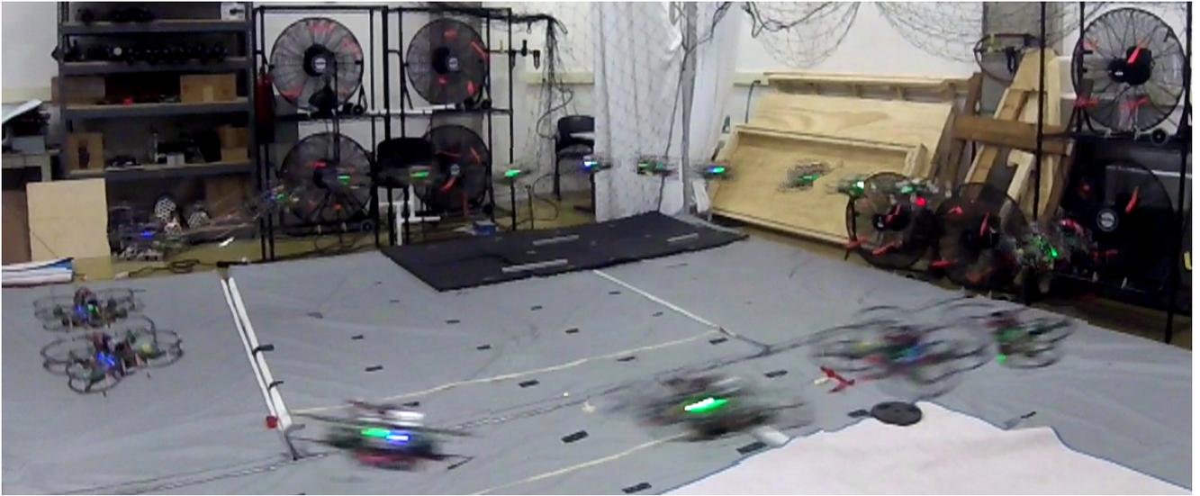
**Figure 17.** Snapshots of quadrotor executing the horizontal circle trajectory in a high-speed, turbulent wind field generated via a set of eight high-power fans
