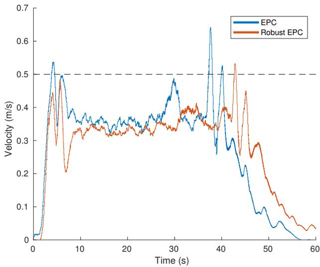
**Figure 24.** Longitudinal velocity profiles for the ground robot running EPC and Robust EPC. The dashed line indicates the enforced constraint bound.
