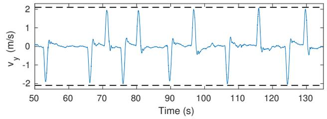
**Figure 30.** Velocity profile for the hexarotor applying Robust EPC. The dashed lines indicate the constraint bounds.
