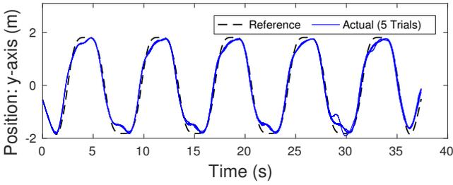
**Figure 10.** Linear trajectory tracking performance across five laps
