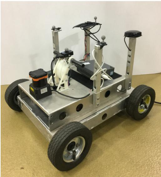
**Figure 21.** The laser-equipped ground robot platform used for experimental validation.
