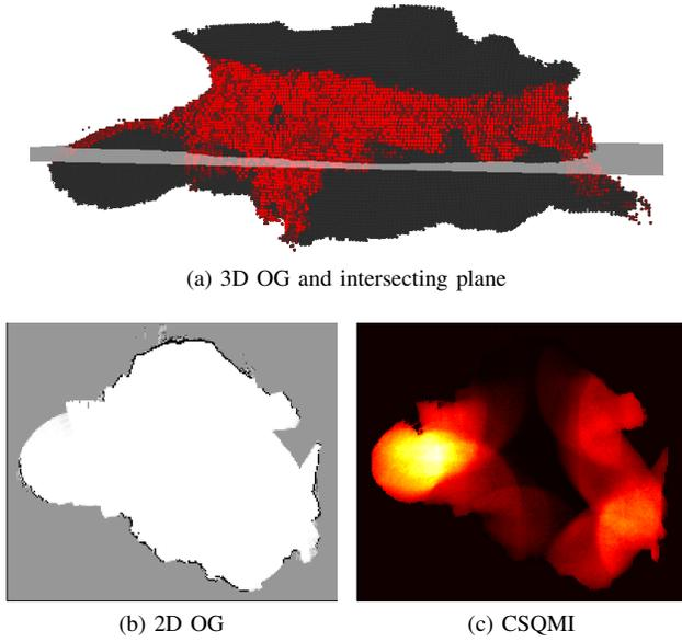
Fig. 4: Illustrative cross-section (a) from the OG shown in Fig. 3 to form a 2D OG (b) with free (white), occupied (black), and unknown (gray) cells. (c) The CSQMI reward is evaluated for a planar sensor at different positions over this cross section to create a heat map (brighter colors corresponding to increased reward). This reward surface is non-smooth and sometimes flat due to occlusions and the limited sensor range.
