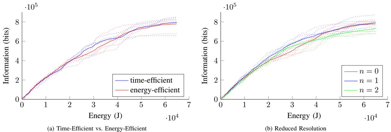
Fig. 6: Information gained (reduction in Shannon entropy) versus time and energy costs. (a) Energy- and time-efficient objectives are roughly equivalent for the operational domain. (b) Evaluation of mutual information on reduced resolution maps leads to improved exploration performance. Dotted lines indicate individual runs and solid lines represent mean values.
