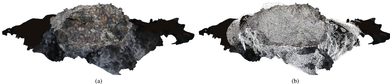
Fig. 7: (a) Angled view of the Indian Tunnel skylight and (b) sensor measurements taken during exploration (shown in white).
