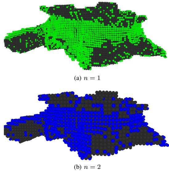
Fig. 5: The OG from Fig. 3 with resolution reduced (a) one and (b) two times. Free cells are dark and occupied cells are colored while unknown cells are not shown.
