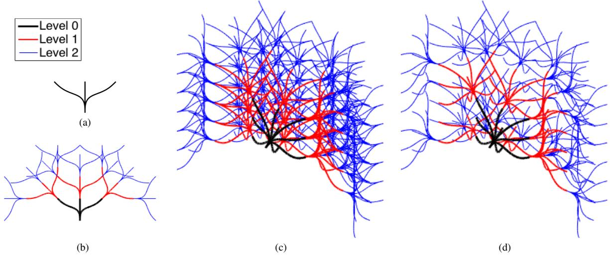
Fig. 2: (a) A dictionary of three motion primitives in 2D. (b) A graph with depth three constructed from the dictionary. (c) A graph in 3D constructed from a dictionary of ten motion primitives (associated dictionary not shown). (d) The graph from (c) after pruning. Sub-optimal and redundant edges are pruned to decrease the number of primitives to search over during exploration.
