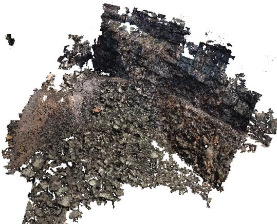
**Figure 14.** A 3d reconstruction from a planned set of images of King's Bowl, using the greedy planning method
