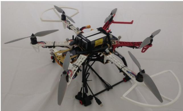
**Figure 25.** The hexarotor platform with a self-contained visual odometry system.
