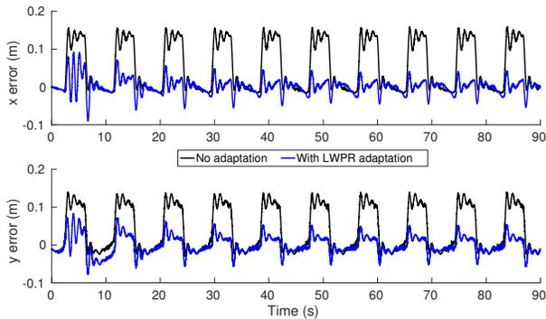
Fig. 4: Comparison of EPC tracking performance with and without LWPR-based adaptation.
