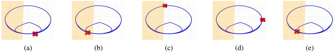
Fig. 1: Snapshots of the quadrotor executing the elliptical trajectory that traverses the disturbance region (highlighted).
