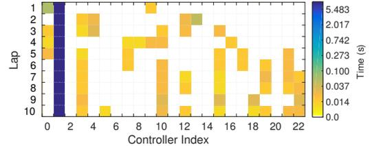
Fig. 2: Learned controllers are reused in subsequent laps, ultimately eliminating the dependence on the intermediate controller (column 0). Colors denote the total usage time (in seconds) for each controller.
