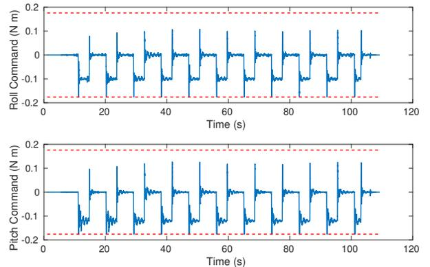
Fig. 3: EPC successfully satisfies roll and pitch control input constraints (dashed red lines) via controller switching.
