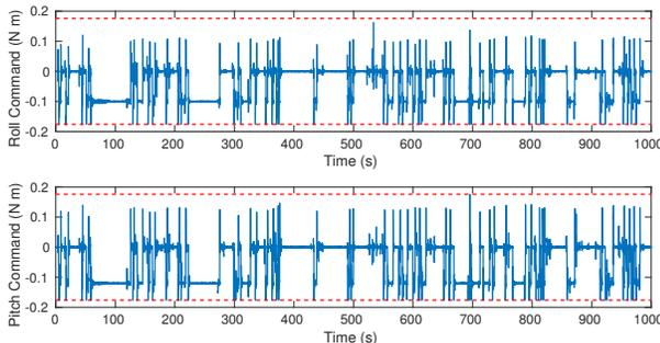
Fig. 10: EPC satisfies control input constraints for the entire duration of the randomized trial while tracking a diverse set of trajectories
