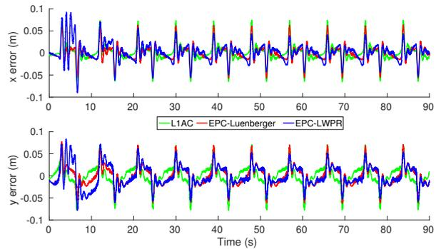
Fig. 6: EPC with LWPR yields improved position tracking error compared to  $\mathcal{L}_1$  adaptive control (L1AC) and EPC with a simple state predictor (EPC-Luenberger).
