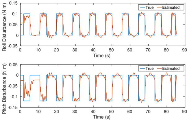
Fig. 5: LWPR accurately estimates the torque disturbances about the  $x$ - and  $y$ -axes as it tracks the elliptical trajectory.
